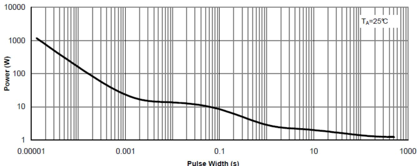
Figure 11: Single Pulse Power Rating Junction-to-Ambient (Note F)
