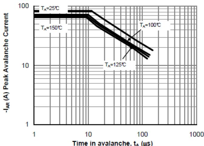
Figure 9: Single Pulse Avalanche capability (Note C)
