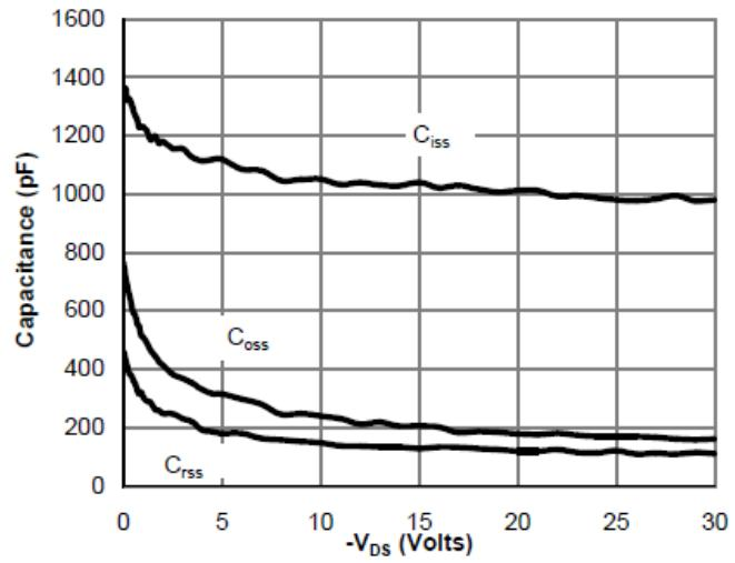
Figure 8: Capacitance Characteristics
