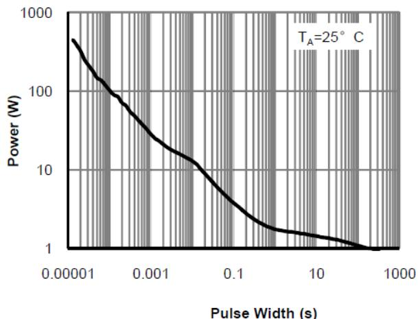
Figure 10: Single Pulse Power Rating Junction-to-Ambient (Note F)
