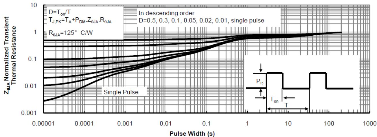
Figure 11: Normalized Maximum Transient Thermal Impedance (Note F)
