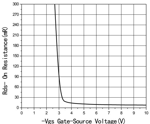
Fig6 Rdson-Gate Drain voltage
