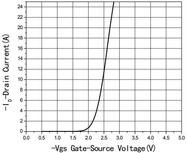
Fig2 Transfer Characteristics
