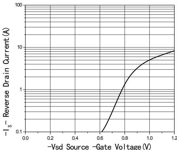
Fig5 Source-Drain Diode Forward
