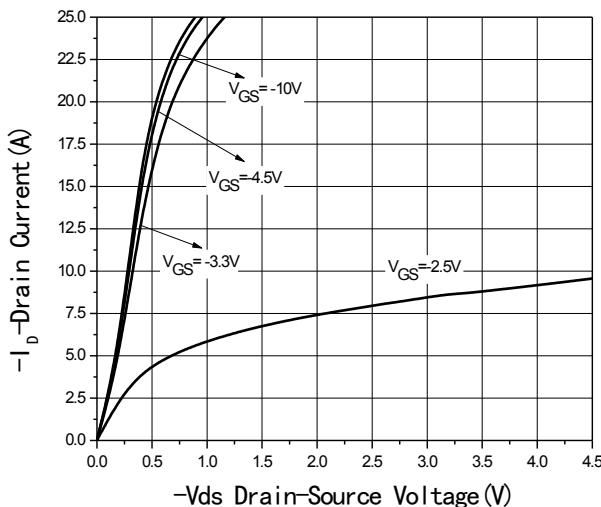
Fig1 Output Characteristics
