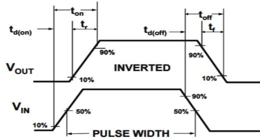
Figure 2: Switching Waveforms
