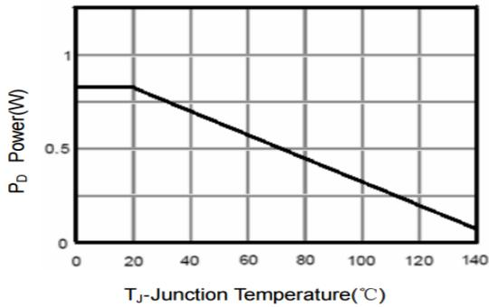
Figure 3 Power Dissipation
