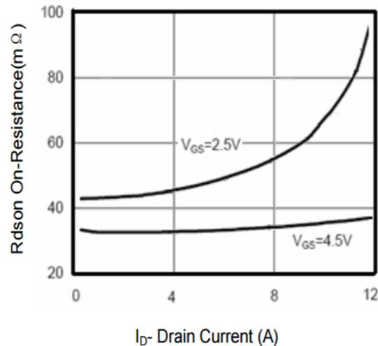
Figure 6 Drain-Source On-Resistance
