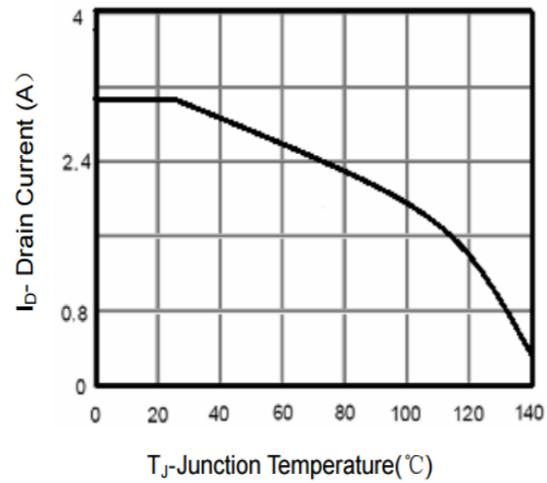
Figure 4 Drain Current
