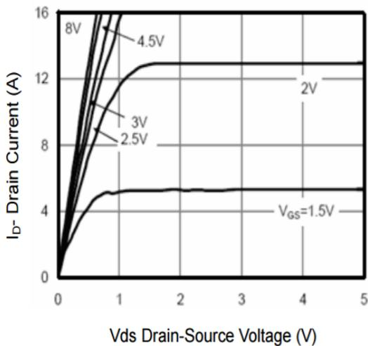
Figure 5 Output Characteristics
