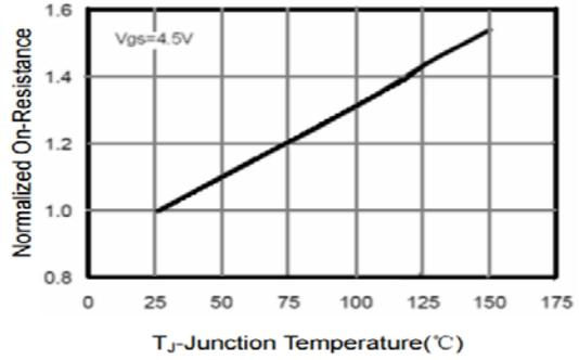
**Figure 8 Drain-Source On-Resistance**
