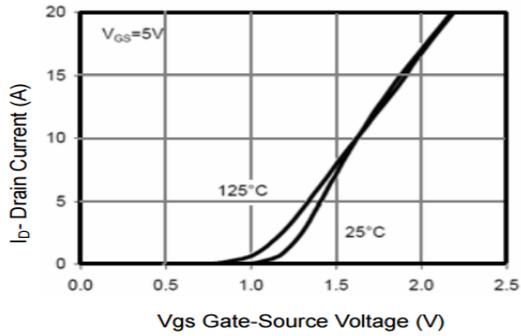
**Figure 7 Transfer Characteristics**
