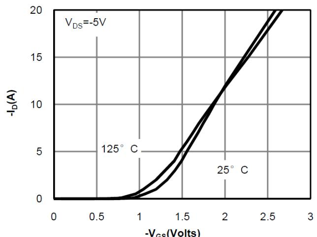
Figure 2: Transfer Characteristics
