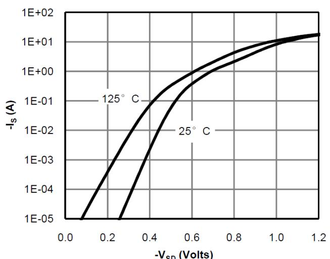
Figure 6: Body-Diode Characteristics
